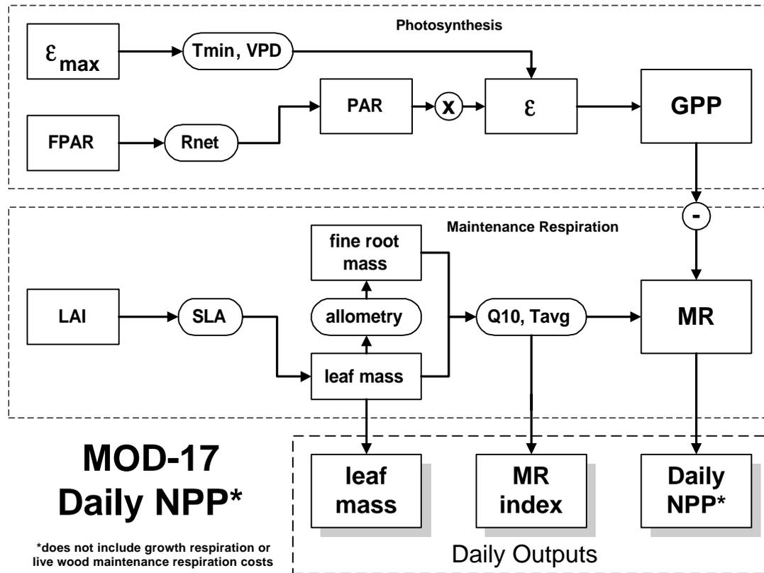
**Figure 3.1** This flowchart illustrates data flow in the daily part of the MOD17 algorithm. Output variables are shown at the bottom, where the notation NPP\* indicates that not all of the autotrophic respiration terms have been subtracted. The remaining terms required to produce actual NPP are handled in the annual timestep.
