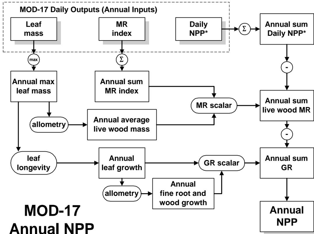
**Figure 3.2** This flow chart illustrates data flow in the annual part of the MOD17 algorithm. Inputs from the daily timestep process are shown at top left. Here the remaining autotrophic respiration terms are taken into account, resulting in an estimate of annual NPP.
