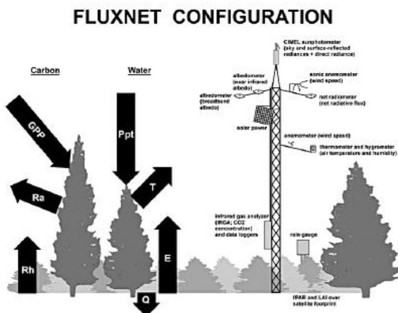
**Figure 6.1.** A generalized FLUXNET tower configuration diagram, showing instrument deployment and key carbon and water fluxes measured. Atmospheric optical measurements, automated surface spectral measurements, physiological process studies, flask sampling and stable isotope sampling are all additions that can be accommodated into this framework to provide a more versatile monitoring system.
